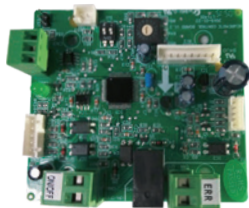
5-core LCAC centralized board
